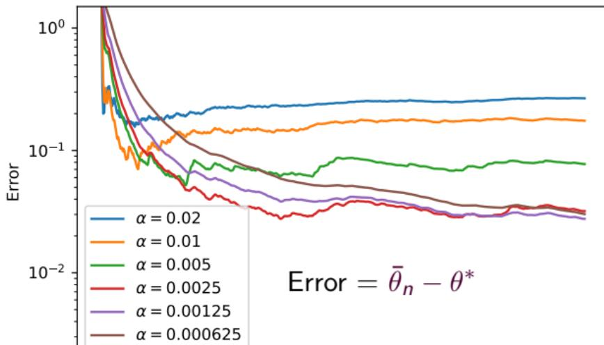
We can extrapolate  $V$  by using two step-sizes  $\alpha$  and  $2\alpha$
