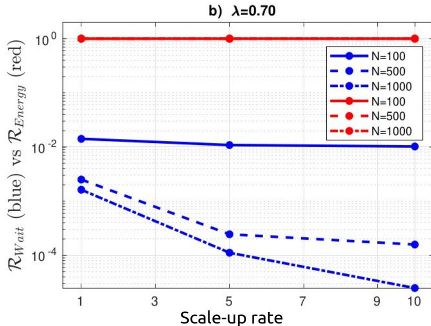
**Possible explanation.** Asynchronous is “proactive”: jobs do not necessarily need to wait any time a scale-up decision is taken.
