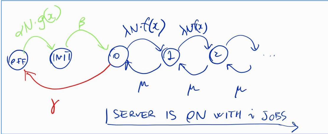
$f(x)$  and  $g(x)$  are the load-balancing and auto-scaling rules
