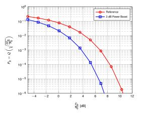
Figure: BER vs. SNR, BPSK, AWGN
