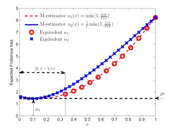
**Fig. 1**: Expected Frobenius loss of the estimator for different u functions as the shrinkage parameter  $\rho$  varies.
