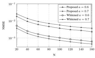
Fig. 3. NMSE of the estimated power versus N with K=1, SNR= 7 dB, N/T=0.5, and c=0.5.
