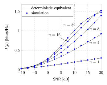
Fig. 2: Mutual Information  $I(\rho)$  versus SNR for different numbers of transmit signatures  $n, N=32, \mathbf{P}=\frac{1}{n}\mathbf{I}_n, L=8$  and  $\alpha=0.5$ .
