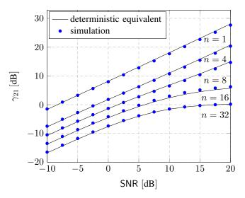
Fig. 3: SINR  $\gamma_{21}$  at the output of the MMSE receiver for different numbers of transmit signatures n, N=32,  $\mathbf{P}=\frac{1}{n}\mathbf{I}_n$ , L=8 and  $\alpha=0.5$ .
