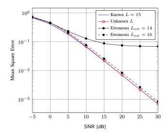
Fig. 2. Mean square error of channel estimate when L=15 is known, known to be in  $\{1,\ldots,32\}$ , or erroneously estimated to  $L_{\rm est}\in\{14,16\}$ ,  ${\rm SNR}=20~{\rm dB},~N=128.$
