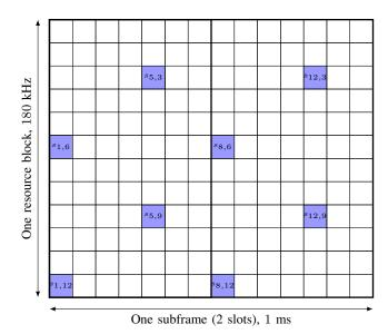
Fig. 1. Time-frequency OFDM grid with pilot positions enhanced
