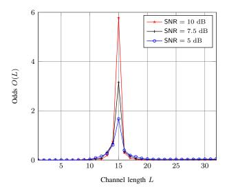
Fig. 3. Inference on channel length O(L) for different SNR, N=128, L=15 (true length),  $L_{\rm min}=32$ ,  $L_{\rm max}=32$
