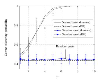
Fig. 4. Comparison of the correct clustering probability between the optimal kernel f(x) (here  $f(x) = \exp(-(x-2)^2)$ ) and the Gaussian kernel  $\exp(-x^2)$ , for different number of observations T per source, using the k-means or EM algorithms. Setting identical to Figure 3.
