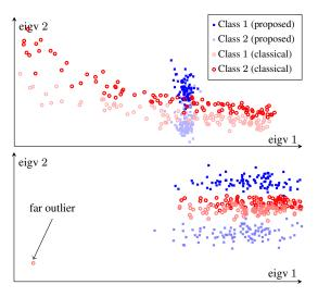
**Fig. 3**. First and second eigenvectors of K for the traditional estimator (red circles) versus the proposed one (blue crosses); (top) random number of snapshots  $n_i$ ; (bottom)  $n_1 = \ldots = n_{m-1} = 512$  and  $n_m = 256$ .
