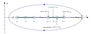
Fig. 2. Integration contour and the logarithm branch cuts.
