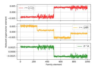
**Fig. 1.** Second dominant eigenvector of  $H_{r_c}$ ,  $H_{\sqrt{\rho(B)}}$ , and  $D^{-1}A$  for  $q_i$  distributed as  $\frac{1}{2}\delta_{0.4} + \frac{1}{2}\delta_{1.6}$ . In this case the  $q_i$ 's,  $i = 1, \ldots, n$ , are sorted in four  $\frac{n}{4}$ -sized consecutive blocks as (1.6, .4, 1.6, .4).
