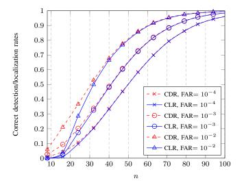
Fig. 9. Correct detection (CDR) and localization (CLR) rates for different levels of false alarm rates (FAR) and different values of n, for drop of variance of  $\theta_1$ . The minimal theoretical n for observability is n = 8.
