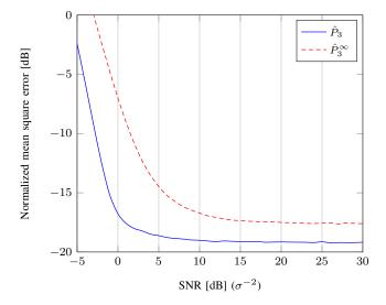
Fig. 6. Normalized mean square error of largest estimated power  $P_3$  for  $P_1=1/16$ ,  $P_2=1/4$ ,  $P_3=1$ ,  $M_1=M_2=M_3=4$ , M=12, N=24, n=128. Comparison between conventional and Stieltjes transform approaches.
