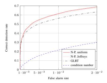
Fig. 8. Receiver operating curve for a priori unknown  $\sigma^2$  of the Neyman-Pearson test (N-P), condition number method and GLRT, N=4, n=8, SNR=  $0~{\rm dB}$ ,  ${\bf h}$  has Gaussian entries of zero mean and unit variance. For the Neyman-Pearson test, both uniform and Jeffreys prior, with exponent  $\beta=1$ , are provided.
