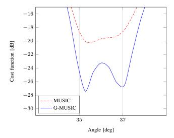
Fig. 7. MUSIC against G-MUSIC for DoA detection of K=2 signal sources, N=20 sensors, n=150 samples, SNR of 10 dB. Angles of arrival of  $35^\circ$  and  $37^\circ$ .
