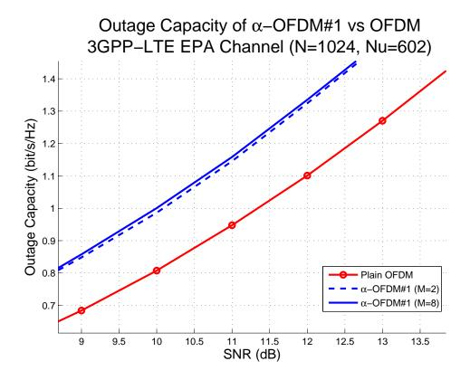
Fig. 3.  $\alpha$ -OFDM#1 Outage Capacity in 3GPP-LTE EPA
