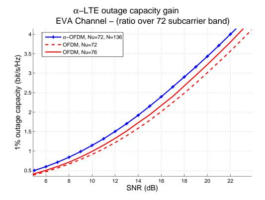
Fig. 6. LTE &  $\alpha$ -LTE outage capacity
