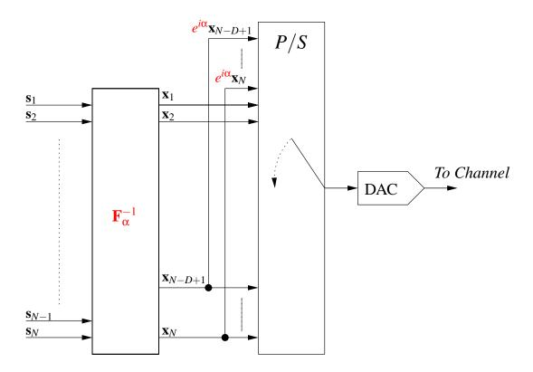
Fig. 1.  $\alpha$ -OFDM transmission scheme
