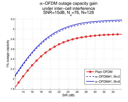
Fig. 5.  $\alpha$ -OFDM#1 with intercell interference
