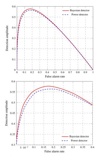
*Fig.* 2. Detection amplitude comparison in MIMO - M = 2, N = 8, L = 10, SNR = -10dB
