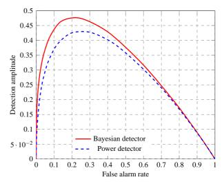
Fig. 1. Detection amplitude comparison in SIMO - M = 1, N = 8, L = 20, SNR = -10 dB
