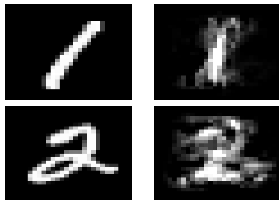
Figure 8.1: Images of digit “1” and “2” from the MNIST database ( left ) and random Gaussian generated from a model with the same mean and covariance ( right ), empirically estimated from all digits of “1” and “2” from the entire MNIST database. Link to code: Matlab and Python
