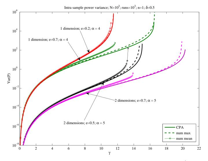
Fig. 4. Plot of the intra sample variance of the power for one- and two- dimensional networks of transmitters of size  $N = 10^3$ , for various values of e. The solid curves are analytically obtained from (70). The meanings of the dashed and starred curves are the same as in Fig. 3(b)
